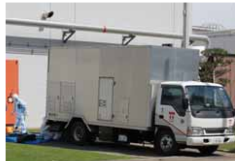
Deploying a power-supply car to the reactor building (Unit 1) Connecting power cables (Unit 1)
